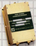
2 Way (90°) Combiner Model QH6031 20-500 MHz 200 W CW
