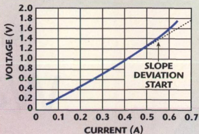
▲ Fig. 4 DC current rating test of the spiral inductor.
